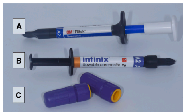
Figure 1. Materials tested. A, Conventional composite resin (C composite) (Filtek Supreme Flowable Restorative; 3M). B, QASi-containing composite resin (Ab composite), (Infinix Flowable Composite; Nobio). C, Amalgam (admix alloy, high copper, nongamma II amalgam; Sphero-don-M, Silmet).
